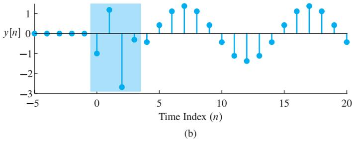
**Figure 6-1:** (a) Input  $x[n] = \cos(0.2\pi n - \pi)u[n]$  and (b) corresponding output  $y[n]$  for the FIR filter with coefficients  $\{1, -2, 4, -2, 1\}$ . The transient region is the shaded area in (b). (Note the different vertical scales.)
