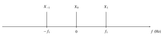
Determine the values for  $f_1$ ,  $X_0$ ,  $X_1$ , and  $X_{-1}$ . Note that the frequencies f are given in Hertz.
