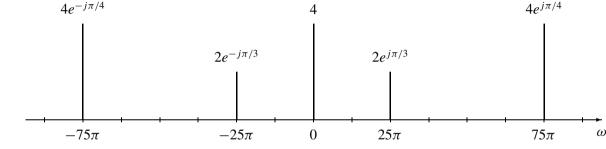
Note that the frequency axis is radian frequency  $(\omega)$  not cyclic frequency (f).
