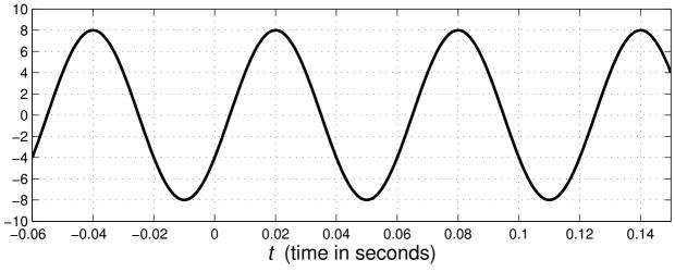
The above graph is a plot of a sinusoidal signal  $x(t) = A\cos(\omega_0 t + \phi)$ .
