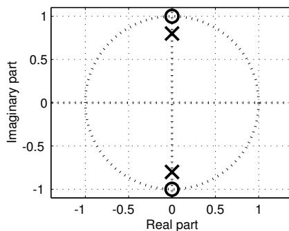
For each of the pole-zero plots (P, Q, R, S), determine which one of the following systems (specified by either an impulse response  $h[n]$ , a difference equation, or a MATLAB statement) matches the pole-zero plot.
