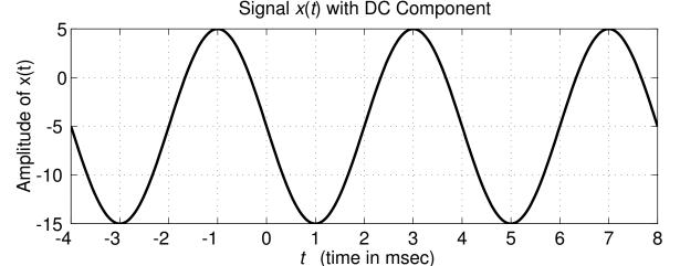
The above signal x(t) consists of a DC component plus a cosine signal. The terminology DC component means a component that is constant versus time.
