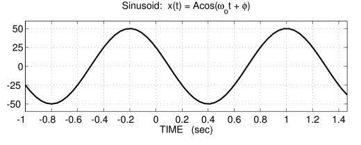
(d) In the figure above determine the frequency ( $\omega_0$ ) in radians/sec. Circle the correct answer. (A)  $5\pi/3$  (B)  $5\pi/6$  (C)  $5\pi/12$  (D) 5/6 (E)  $2.4\pi$
