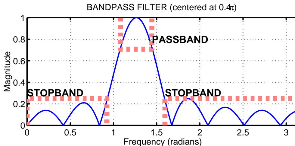
Figure 3: Passband and Stopband for a typical FIR bandpass filter. In this case, the maximum value is 1, the passband is the region where the frequency response is greater than  $1/\sqrt{2} = 0.707$ , and the stopband is defined as the region where the frequency response is less than 25% of the maximum.
