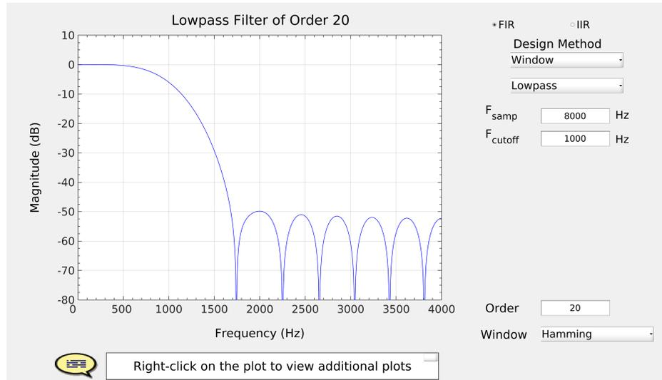
Figure 1: Interface for the **filterdesign** GUI. When the Filter Choice is set to FIR, many different window types can be selected, including the Hamming window and the Rectangular window (i.e., no window). The specification of one or more cutoff frequencies ( $f_{co}$ ) must be entered using continuous-time frequency (in Hz), along with a sampling rate ( $f_s$ , also in Hz). In normalized frequency, the cutoff frequency is  $\hat{\omega}_{co} = 2\pi(f_{co}/f_s)$ .
