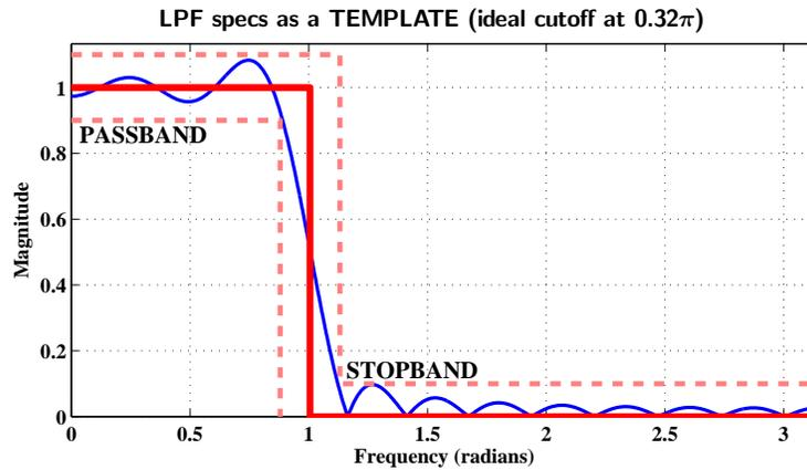
Figure 3: Tolerance scheme drawn around an ideal LPF with a cutoff frequency of  $\hat{\omega}_c = 0.32\pi$ . Dashed lines indicate the maximum allowable deviation from the ideal LPF. The template uses  $\hat{\omega}_p = 0.28\pi$ ,  $\hat{\omega}_s = 0.36\pi$ , and  $\delta_p = \delta_s = 0.1$ . The actual FIR filter shown is the length-23 FIR filter from Fig. 2 which just barely meets these specs.
