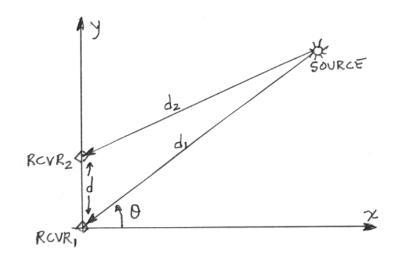
Figure 1: Source with two receivers. The angle  $\theta$  is shown as positive, but  $\theta$  could be negative if the source lies in the fourth quadrant. When  $\theta > 0$  the signal arrives first at receiver #2. The two receivers on the *y*-axis cannot distinguish left from right, so we *assume the source does not lie in the second or third quadrants*.
